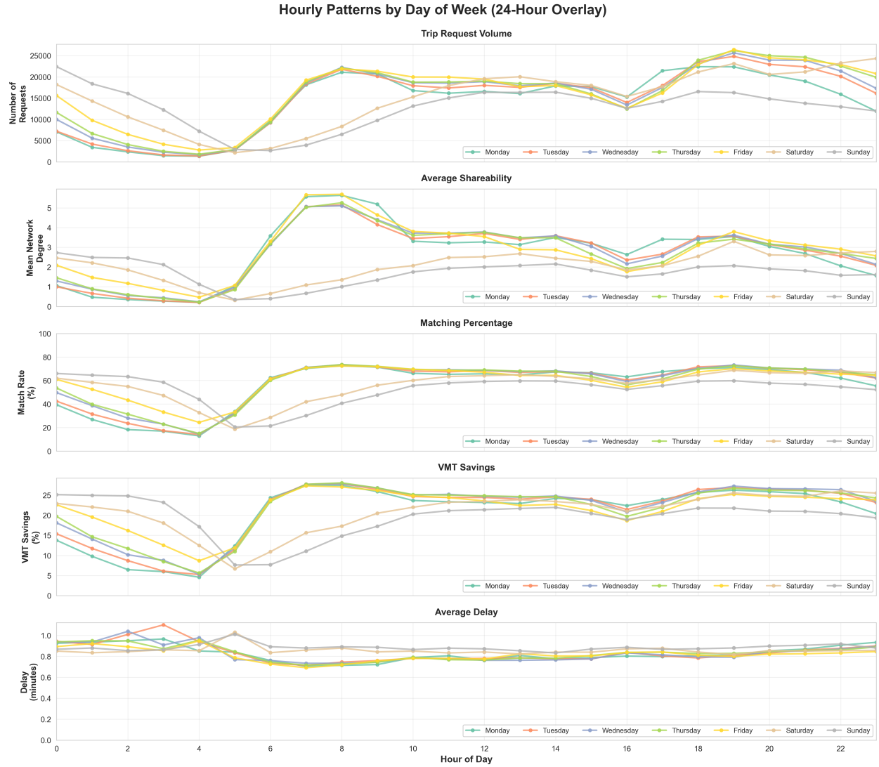
Figure 1: Hourly patterns by day of week (June 3–9, 2013). Each line is a day; panels show demand (top), shareability, match rate, system-wide VMT savings, and average delay.
